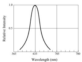
Fig.1 RELATIVE INTENSITY VS. WAVELENGTH
